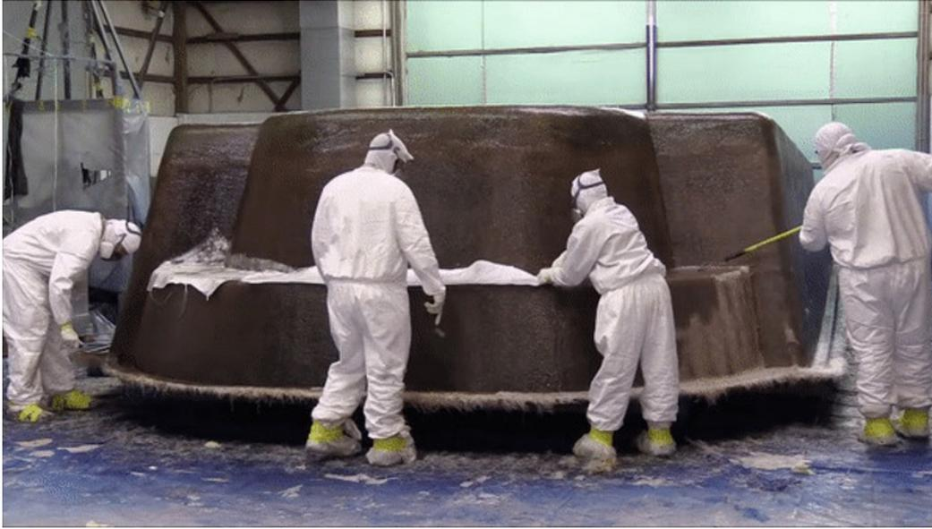
We reinforce areas subject to the most bending stresses -- primarily where the shell transitions from a flat surfaces (floors) to upright (walls) -- with a **layer of woven roving fiberglass** for additional strength.
