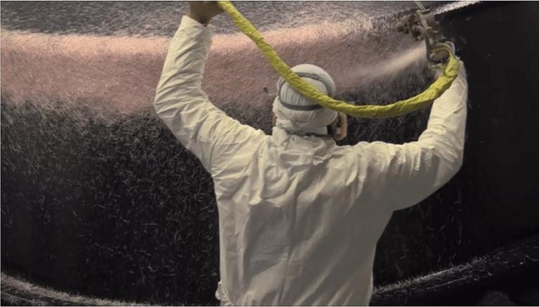
After applying the gelcoat surface and adding vinyl ester for corrosion and blister resistance, we focus on building strength into the pool shell with chopped fiberglass. We apply this material with a “chopper gun” that cuts long strands of glass fiber into pieces about an inch long. The gun also sprays resin and catalyst onto the mold while it chops fiberglass. Once chopped and sprayed, we roll out the fiberglass layer to strengthen it and remove any potential air bubbles.
