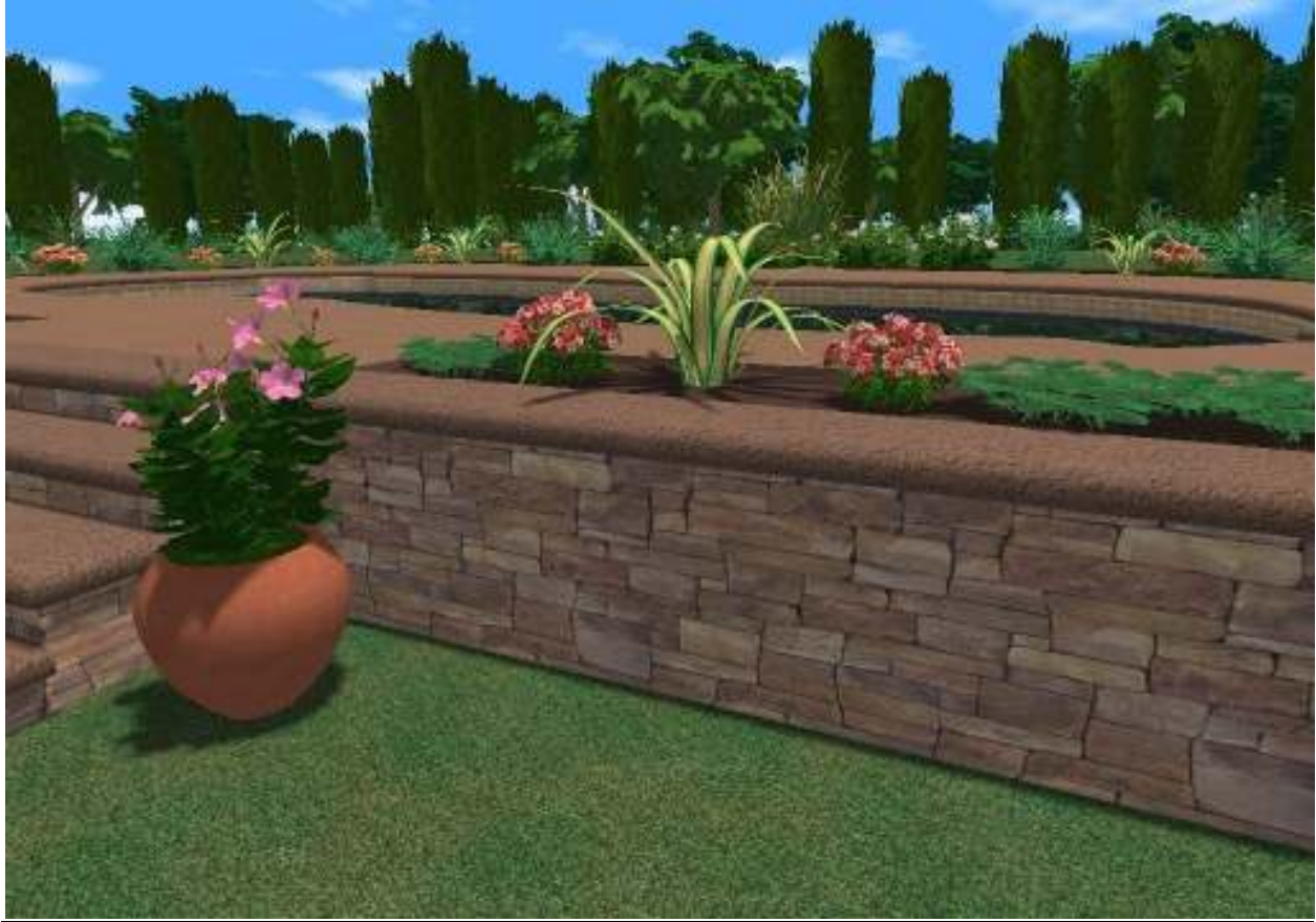
Natural stone retaining wall with concrete cap
